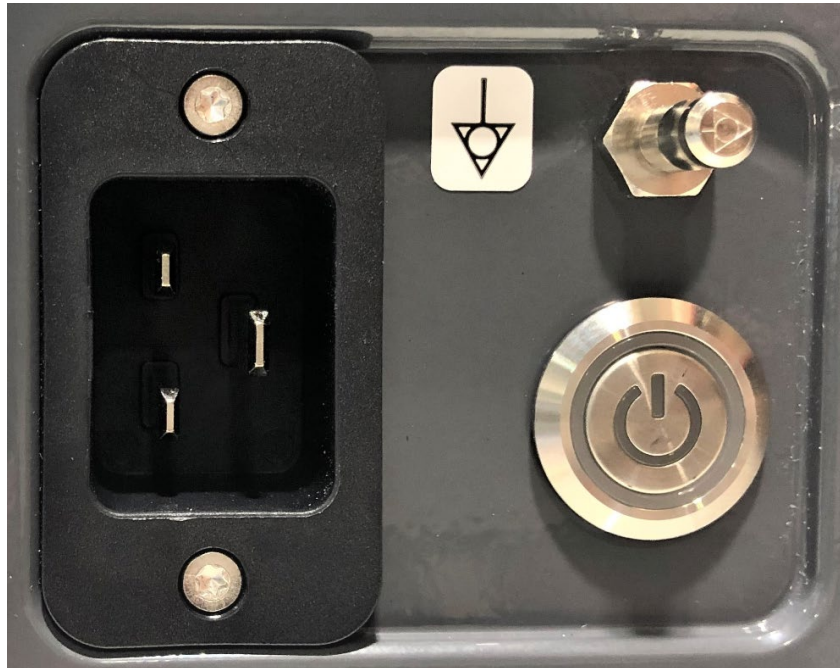
Figure 18 – Mains Power Supply (1)
