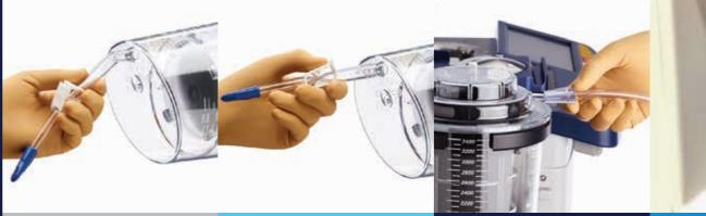
Place the collection reservoir into the reservoir holder. Attach a vacuum line to the yellow-capped port on the collection reservoir.
